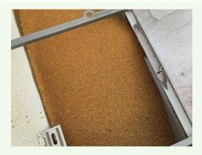
It's common to see some small trash on top of truck sample around the edge as shown to the left, this is a good sample.
